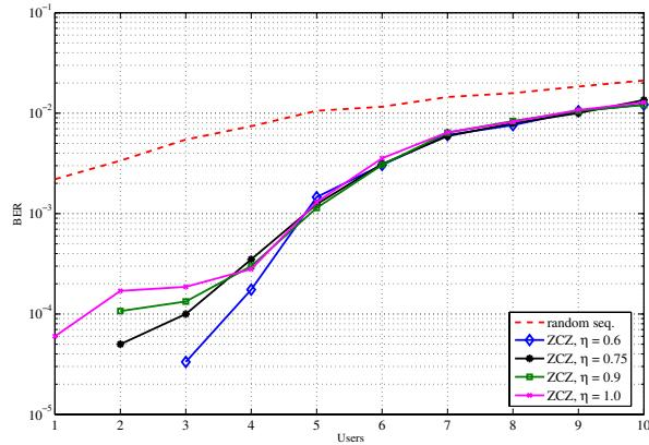
Fig. 6. Proposed receiver performance, parameterized by  $\eta$ . Uplink,  $N = 32$ .
