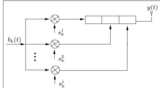
Fig. 2. Illustration of the spreading structure, for the user  $k$ .
