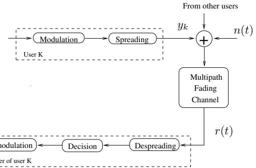
Fig. 1. Block diagram of the system model
