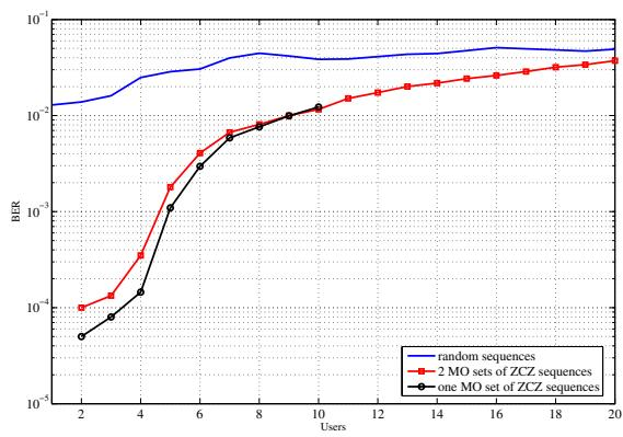
Fig. 4. Proposed receiver performance for three different schemes. Uplink,  $N = 32$  and  $\eta = 0.75$ .
