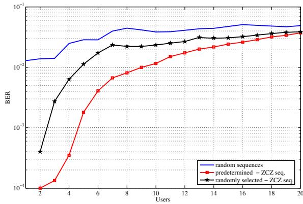
Fig. 5. System performance analysis for three different sequences selection. Uplink,  $N = 32$  and  $\eta = 0.75$ .
